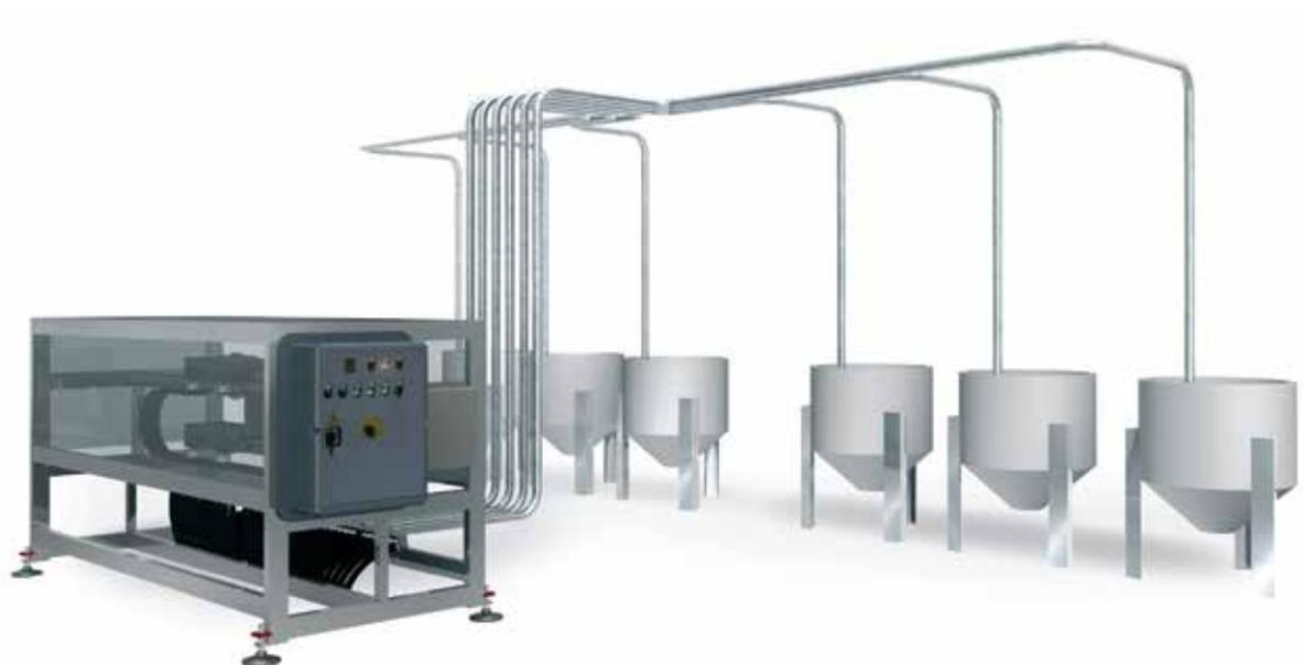
The multiple line distribution system is a Color Service creation and for two decades has proved to be the most secure system for feeding products to different services. The plant has a pipe system for each destination. All the piping is hooked up to the distribution head plate with a mobile arm that couples onto on the selected output to pump the liquid to destination.
