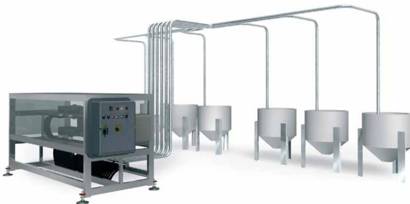
The multiple line distribution system is a Color Service creation and for two decades has proved to be the most secure system for feeding products to different services. The plant has a pipe system for each destination. All the piping is hooked up to the distribution head plate with a mobile arm that couples onto on the selected output to pump the liquid to destination.
